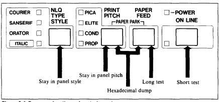
Figure 2-4. Power-up functions of control panel
