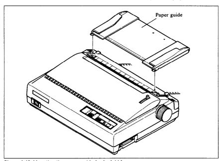
Figure 1-12. Mounting the paper guide for fanfold forms
