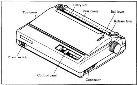
Figure 1-2. The printer's external parts
