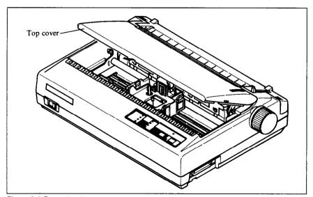
Figure 1-4. Removing the top cover
