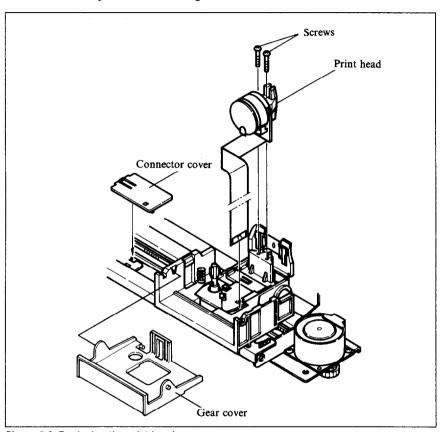
Figure 5-2. Replacing the print head
