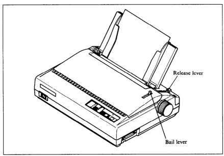
Figure 1-8. Loading a single sheet
