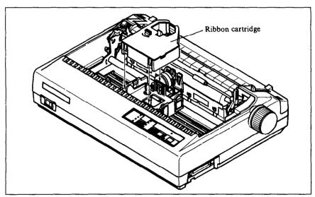
Figure 1-5. Installing the ribbon cartridge
