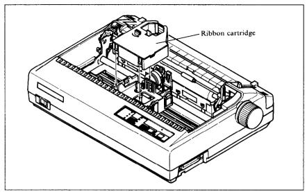
Figure 5-1. Replacing the ribbon cartridge
