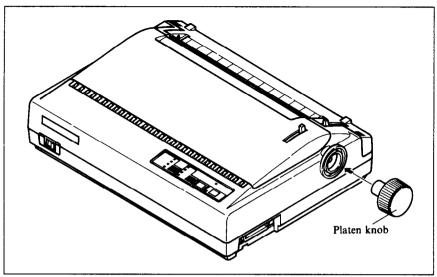
Figure 1-3. Mounting the platen knob
