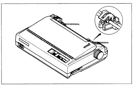
Figure 1-11. Closing the sprocket covers
