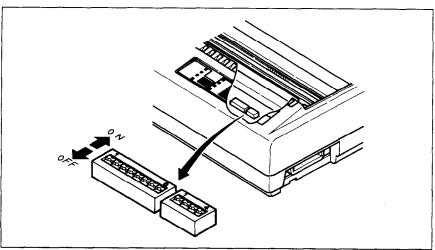
Figure 1-15. DIP switches
